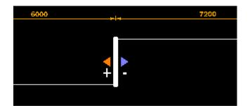
15. Input "-1000" in the *Shift* text box. The colour of the blue arrow indicates that a negative value will shift the line right 1000mm.
