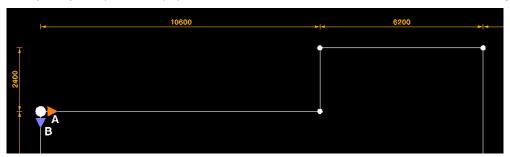
18. In the Cutout text box, type "1100 9700". This will cut out a rectangle 1100mm in the orange direction and 9700 in the blue direction. The plan should now match the example drawing.
